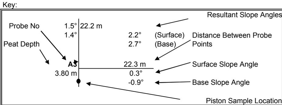
Note: Negative slope angles indicate ground surface/base slopes opposite to overall slope direction.
