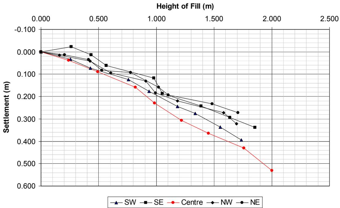
Figure No. 4 – Settlements recorded during the road test
