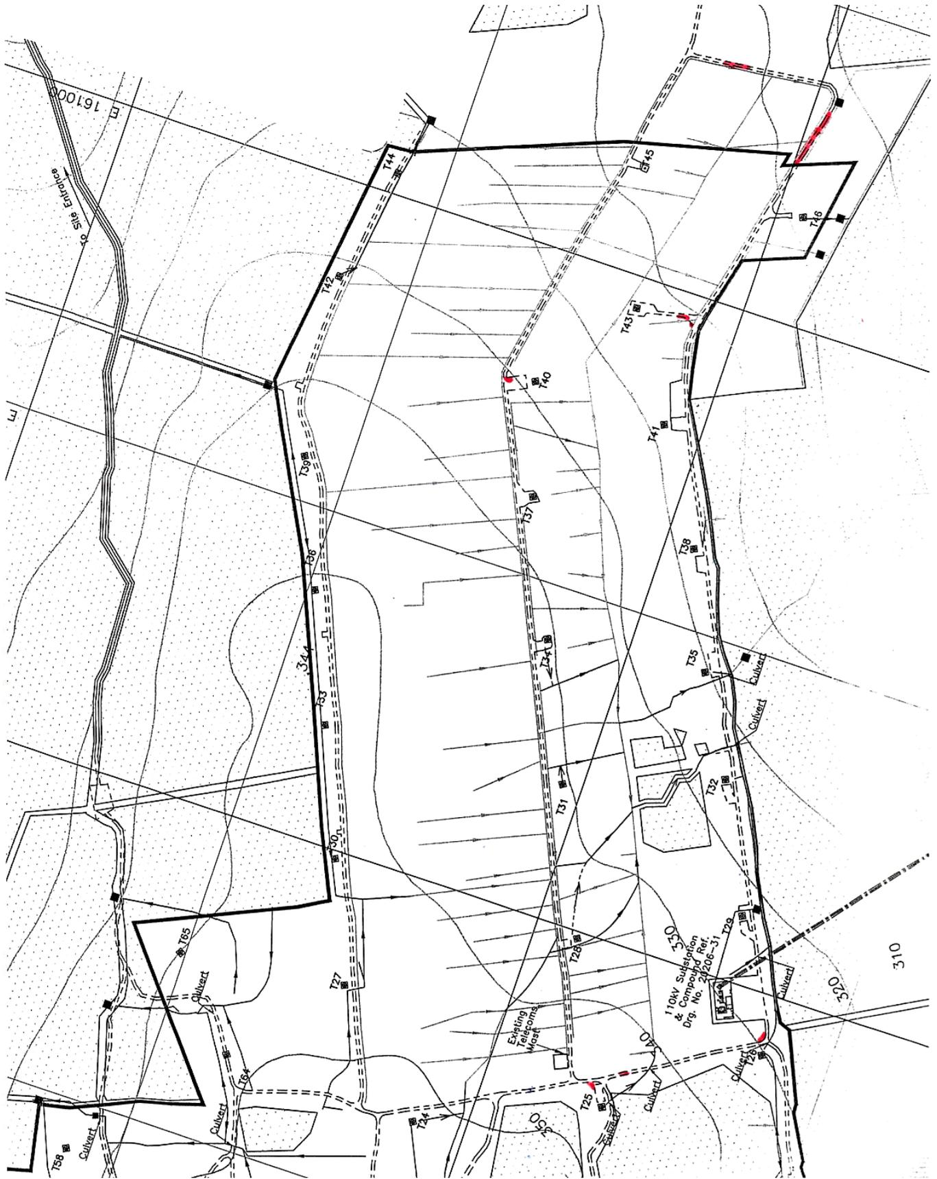
Figure No.3 – Sections of floating road classified as poor on east side of site (marked in red)
