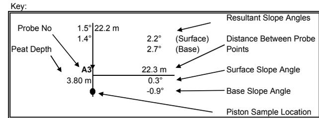
Note: Negative slope angles indicate ground surface/base slopes opposite to overall site direction.
