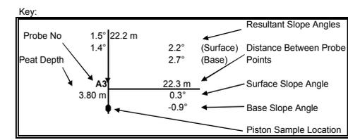
Note: Negative slope angles indicate ground surface/base slopes opposite to overall slope direction.
