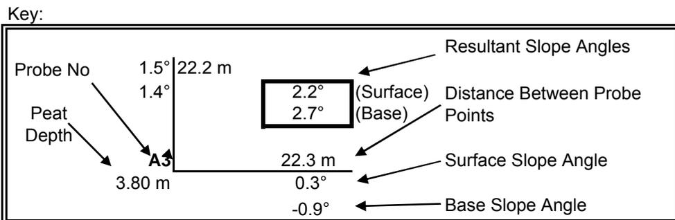
Note: Negative slope angles indicate ground surface/base slopes opposite to overall slope direction.
