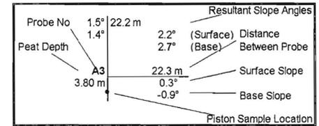
Note: Negative slope angles indicate ground surface/base slopes opposite to overall slope direction.
