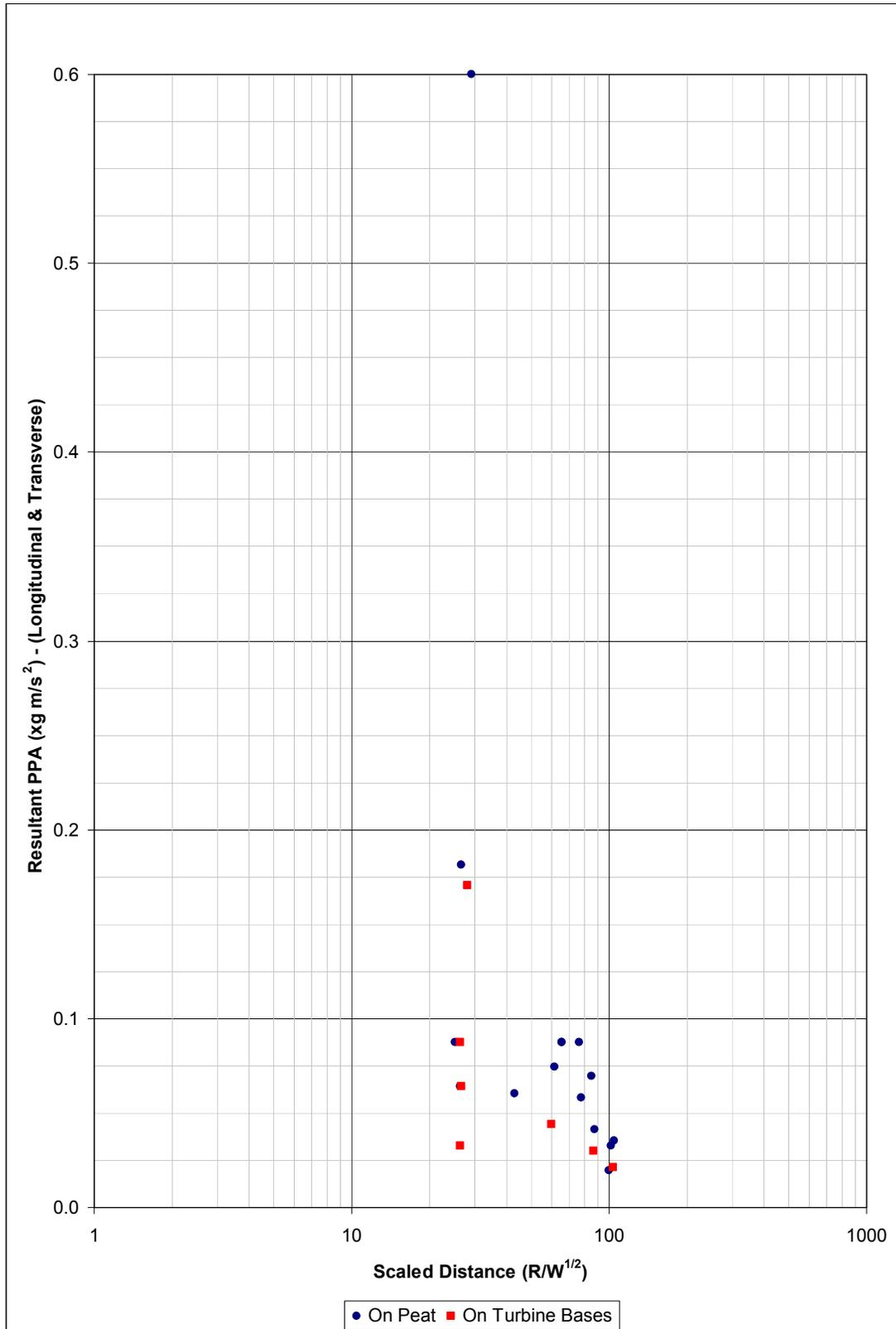
Figure No.2 – Plot of PPA vs Scaled Distance for blasts in Borrow Pit No.2
