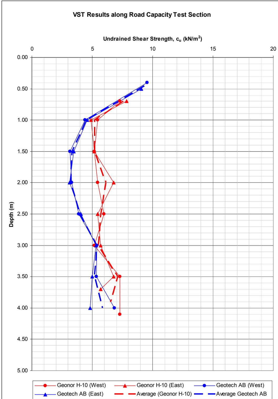
Figure No.2 – Vane shear test results
