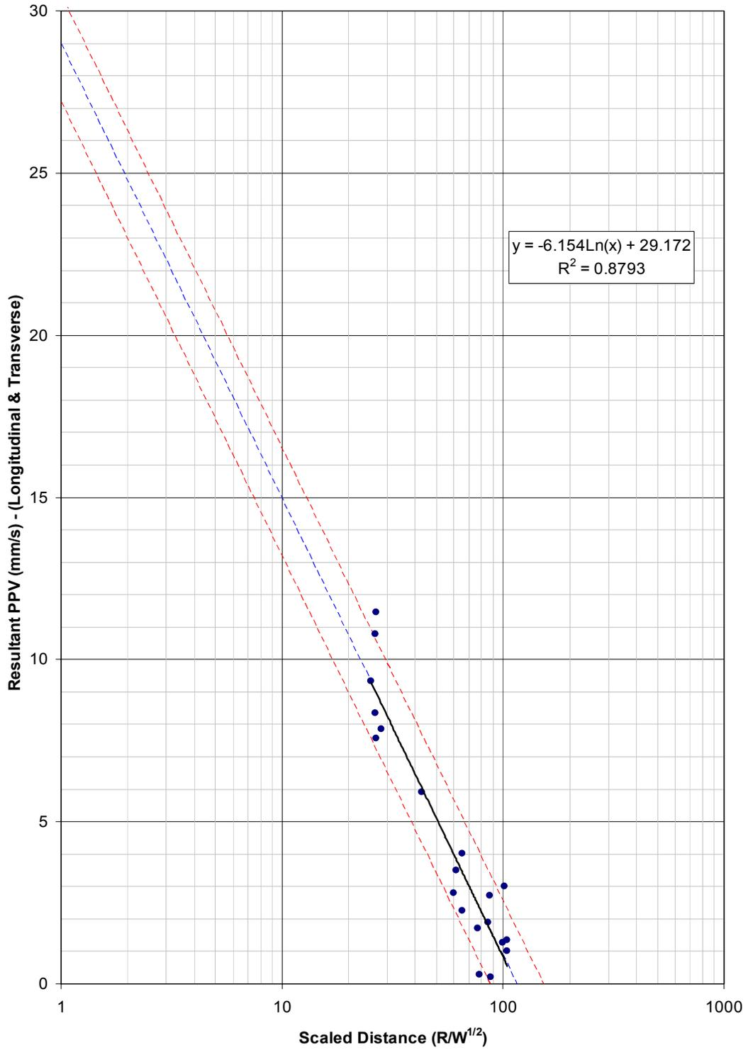
Figure No.3 – Best-fit trend line through resultant horizontal PPV data
