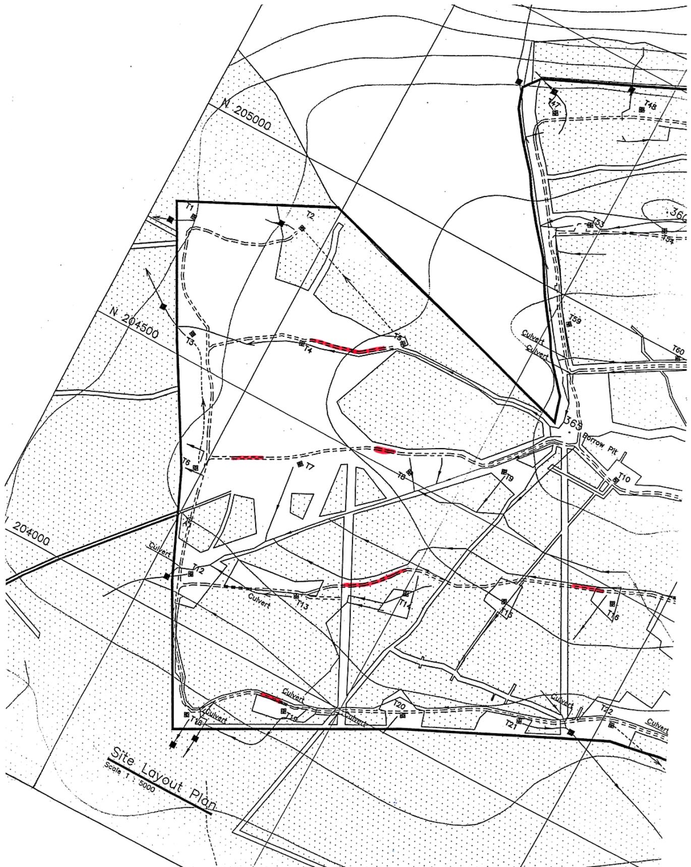
Figure No.1 – Sections of floating road classified as poor on west side of site (marked in red)
