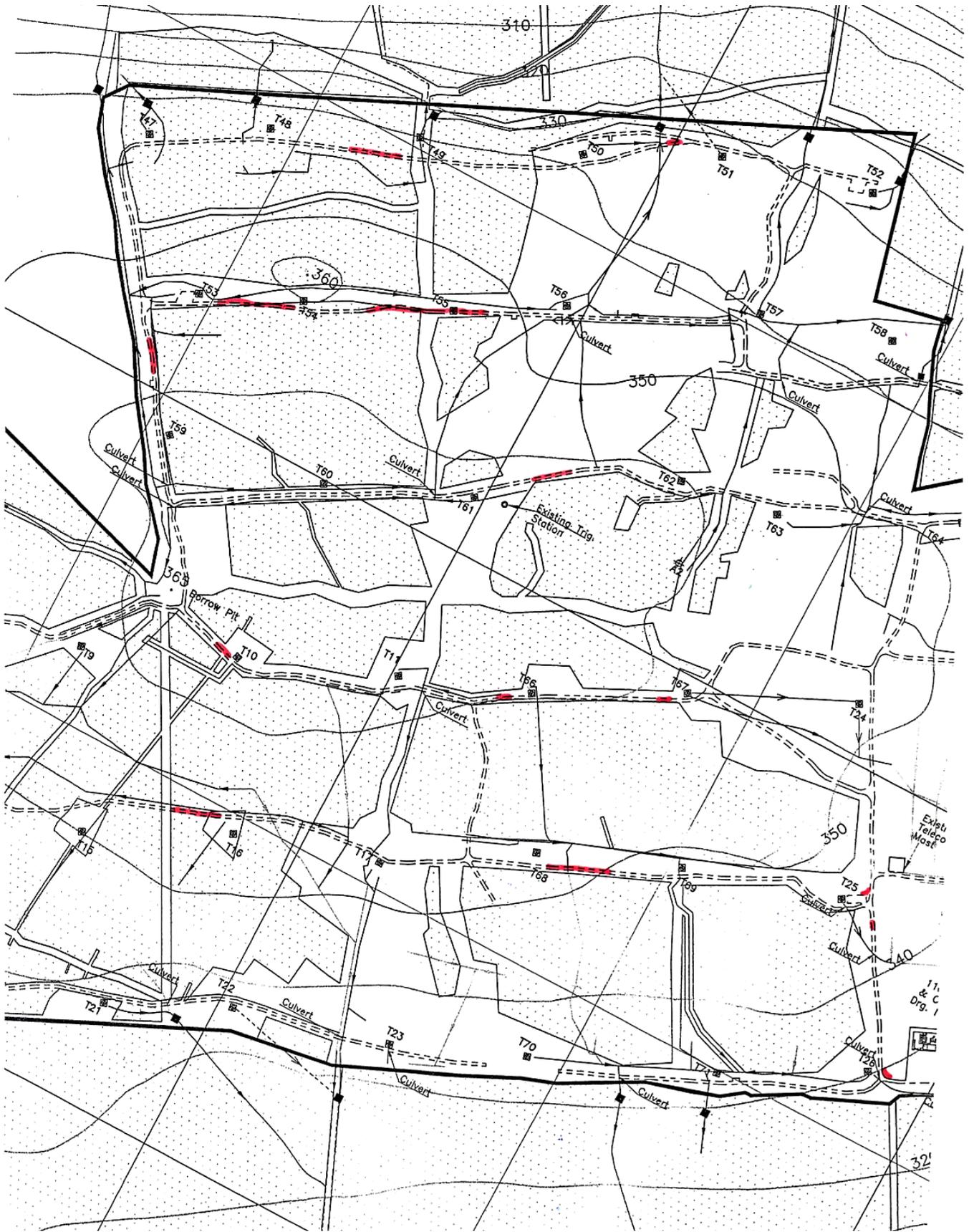
Figure No.2 – Sections of floating road classified as poor in central section of site (marked in red)
