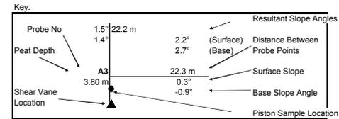
Note: Negative slope angles indicate ground surface/base slopes opposite to overall slope direction.
