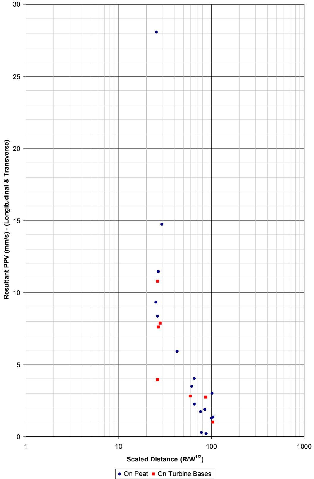
Figure No.1 – Plot of PPV vs Scaled Distance for blasts in Borrow Pit No.2
