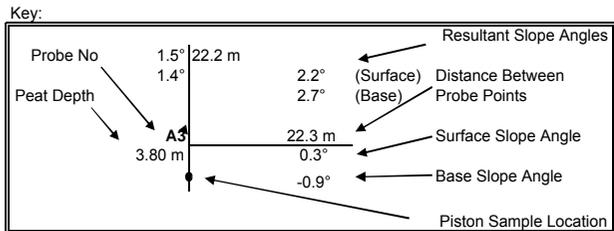
Note: Negative slope angles indicate ground surface/base slopes opposite to overall s
