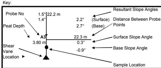
Note: Negative slope angles indicate ground surface/base slopes opposite to overall slope direction.
