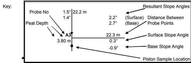
Note: Negitave slope angles indicate ground surface/base slopes opposite to overall slope direction.
